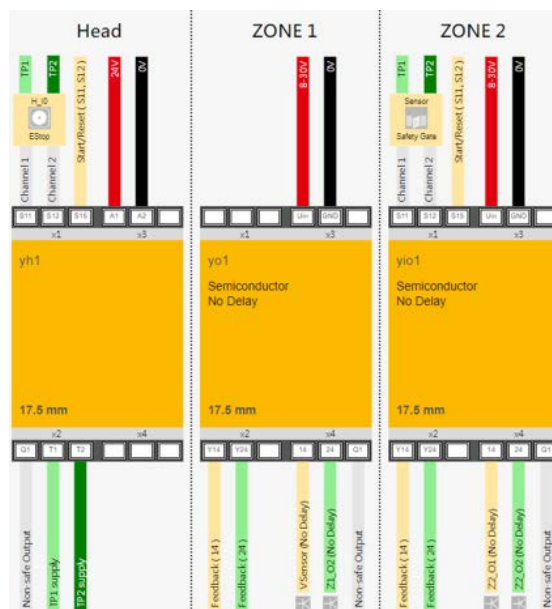
Figure 15 - Connection diagram myPNOZ with semiconductor outputs
