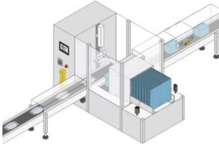
Figure 1 - Layout of cardboard feed
