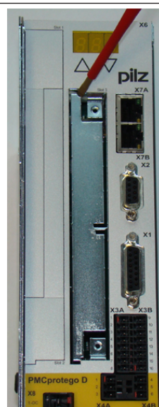
3. Break the top link and lever out the cover plate
