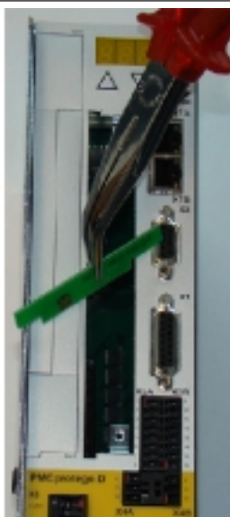
4. Use suitable pliers, pull out the blank in the safety module plug
