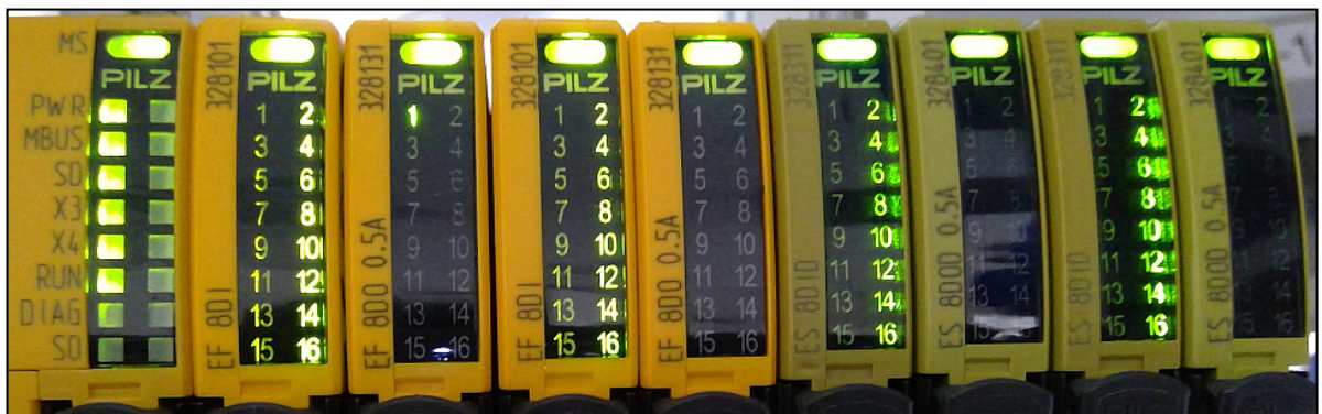
Figure 67: PSS u2 – Diagnostic status with error-free configuration
