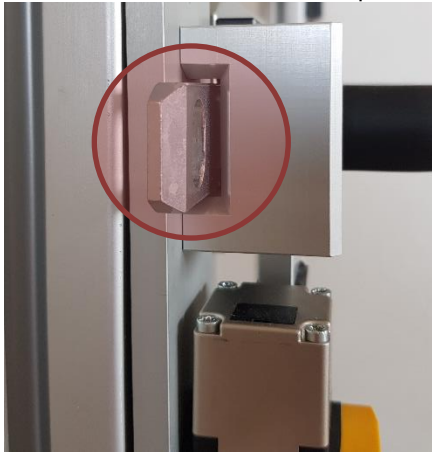
Figure 4: Robust bolt and bolt-seat
