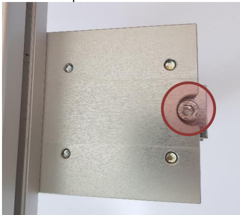
Figure 7: Extended bolt stop
