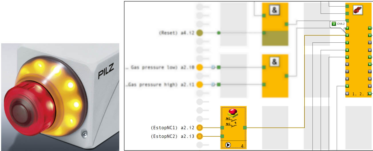
Figure 29: PNOZmulti program – Element 'Emergency stop'
