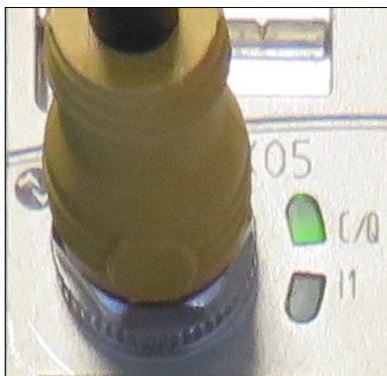
Figure 88: PDP67 – Activation of the IOLS ports » Port 1 (X05)
