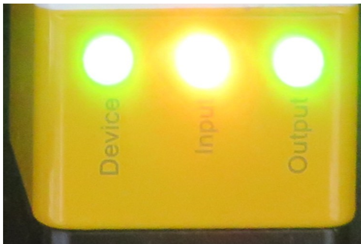
Figure 95: Pilz PITgatebox – IO-Link safety status » 'Device' LED
